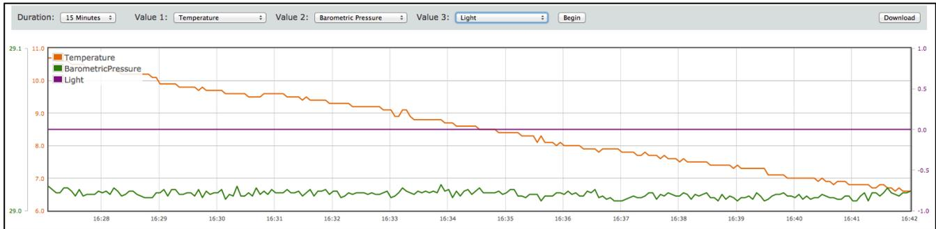
To change the graph, select the desired value or values and duration using the drop down boxes, then press Begin. To save the current graph data, click the Download button to the upper right of the graph. This saves the graph data in comma-separated format, with headers and other identifying information.
