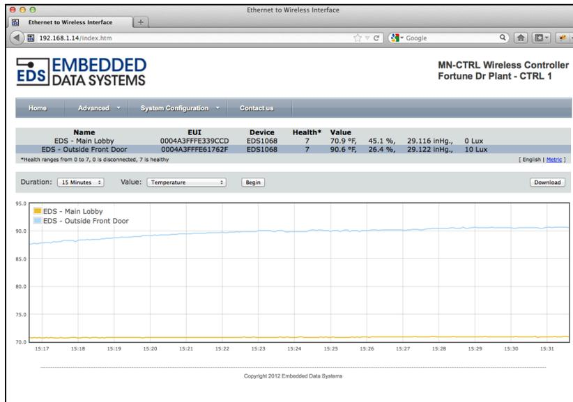
The device page for the EDS1068 is shown here. This sensor measures temperature, humidity, barometric pressure and light, has a discrete input with pulse counter and activity latch, plus an optional relay output. Similar display features apply to all device pages.
