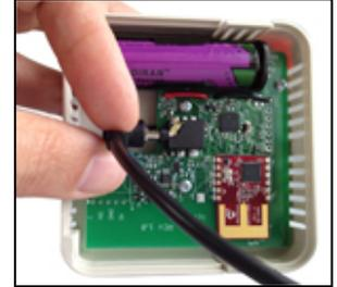
2. **Apply power to the MeshNet Controller a second time.** The green PWR/ACT LED located on the front of the Controller will begin to flash at one-second intervals, indicating that the product is operating normally. Power must be 5 volts +/- 10% at 400 milliamp.
